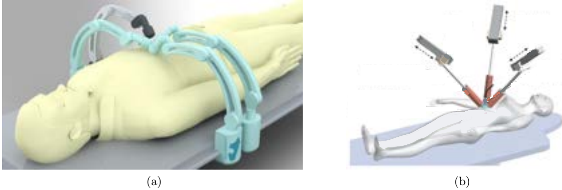
Figure I.12: Examples of magnetic manipulation systems with moving electromagnets: (a) the robot-assisted magnetic manipulation proposed by Véron et al. [130], and (b) the DeltaMag system consisting of three parallel mobile coils [131].
