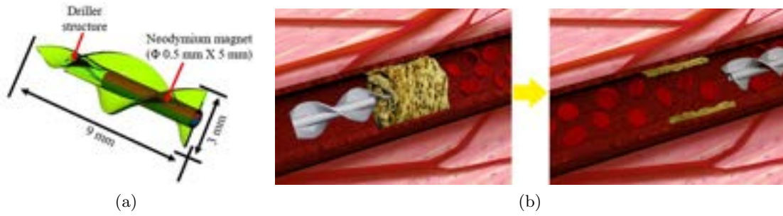
Figure I.8: Drilling microrobot: (a) fabrication procedure of the magnetic drilling actuator; (b) conceptual schematic of the designed microrobot as an intravascular driller in a 3D vascular network. [37]
